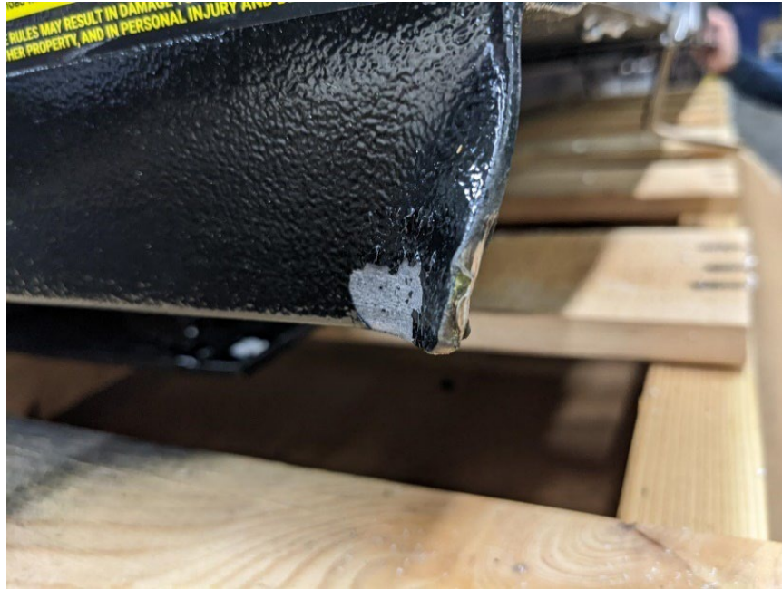
Figure 2-Example of Damage, Bent Corner
